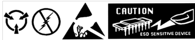
FIGURE 8-8 Symbols indicating ESD sensitivity
