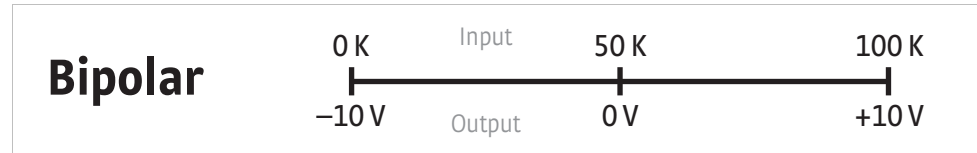
FIGURE 5-3 Analog output with polarity set to bipolar
