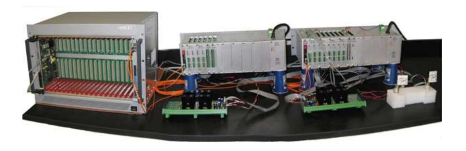
Turbo PMAC2-VME UltraLite connected by optical fibers with two UMAC MACRO chassis
