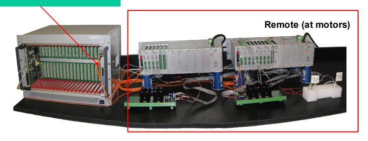
Turbo PMAC2-VME UltraLite connected by optical fibers with two UMAC MACRO chassis. There is also a PCI version that may be supported with EPICS-3.14 and same set of EPICS DB.
