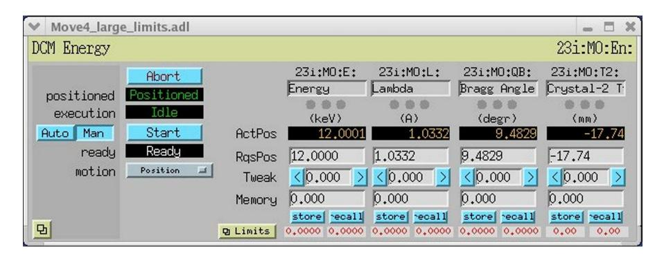
An example of the MEDM screen for monochromator energy assembly
