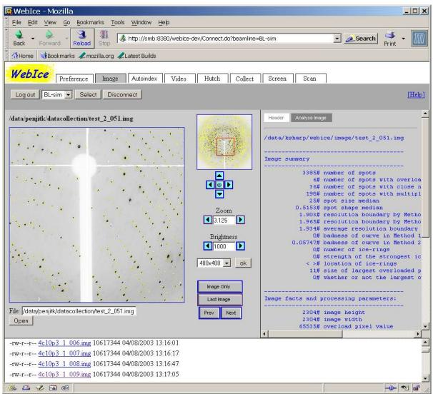
Image Viewer also enables the user to analyze last collected image from beam line with an in-house program called Spotfinder.
